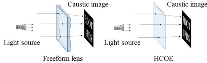
Fig. 1. Caustics images using (a) conventional freeform lens and (b) holographic caustic optical elements.
